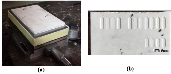
Fig. 8. (a) Machining setup (b) Machined slots
