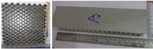
Figure 3 Honeycomb Core sandwich structure
