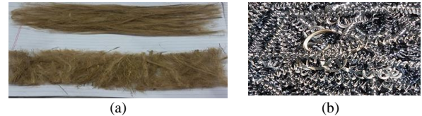
Fig. 2. (a) Jute (upper) and coir (below) fibres in un-treated condition, (b) Metal scrap in form of chips from drilling
