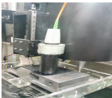
Fig.1 Laser Confocal Chromatic Sensor integrated with the BEMRF setup [14]
