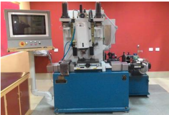
Fig. 3 FSW machine set-up
