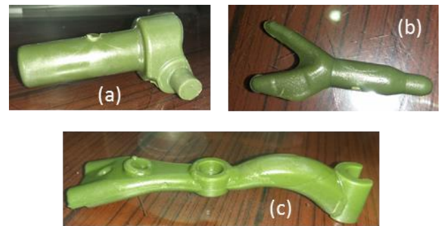
Fig. 6. Wax models for investment casting of (a) Joint, (b) Fork yoke, and (c) Fork
