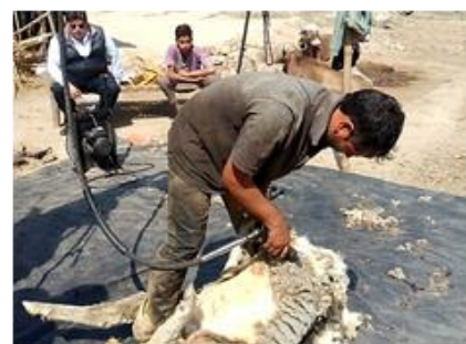
Fig. 7. Trials of indigenous motor, improved flexible drive and handpiece with comb and cutter
