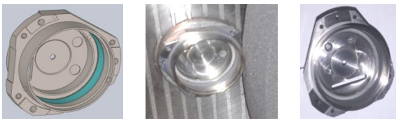
Fig. 6: Main Body (CAD model, Grinding set-up and Hardware respectively)
