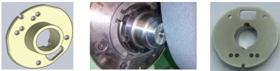
Fig. 2: Magnetic Body (CAD model, Grinding set-up and Hardware respectively)
