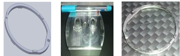
Fig. 4: Spring (CAD model, Fixture set-up and Hardware respectively)
