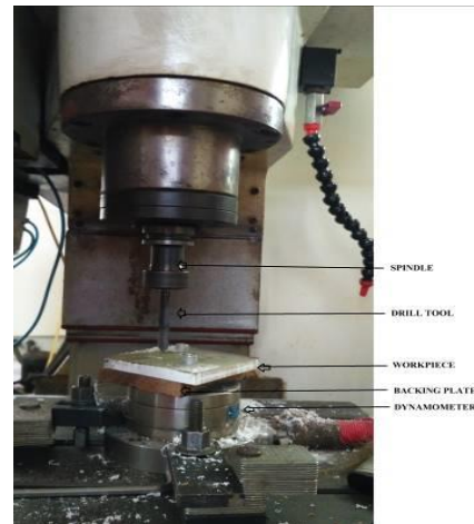
Figure 1 CNC Drilling Machine set up (with dynamometer)
