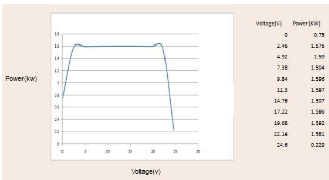
Fig. 6. Simulation result of Peltier module
