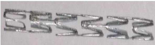
Fig. 11. Stent prototype fabricates using PCM
