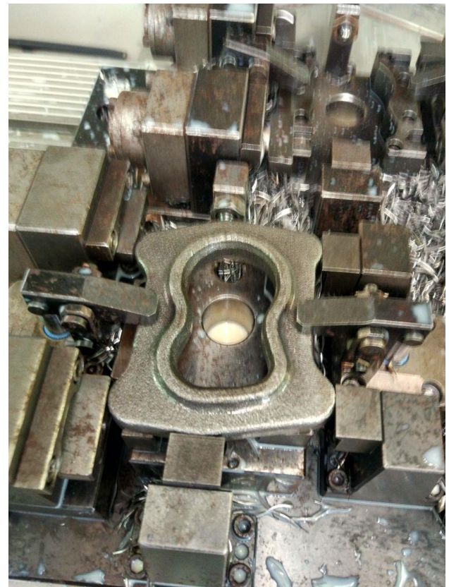
Fig. 6. Photograph of manufactured fixture
