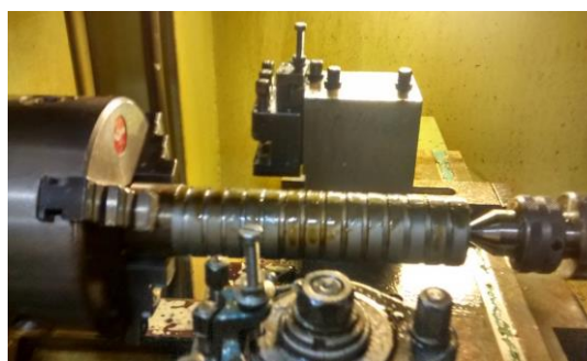
Fig-4 Finishing operation in Schaublin 125CCN CNC lathe
