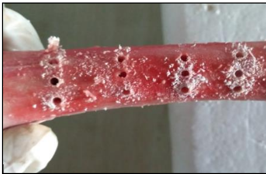
Fig. 2. Femur bone pre-drilled for thermocouple insertion
