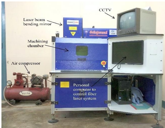
Fig. 1 Photographic view of the multi diode pumped pulsed fiber laser system
