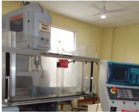
(c) CNC milling used for machining the tooling.
