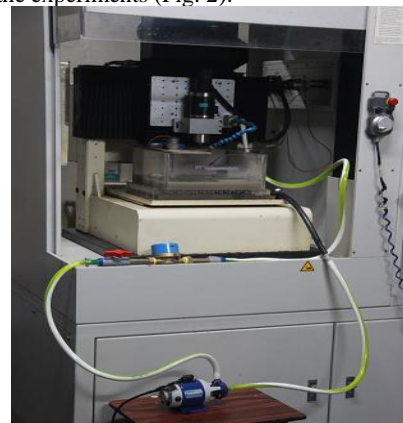
Fig. 2 External Dielectric Circulation setup
