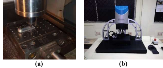
Fig.4. Experimental setup (a) Micro machining centre (b) 3D Optical profiler
