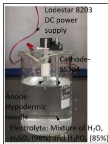
Fig. 4. Experimental set up for electropolishing the Hypodermic needle
