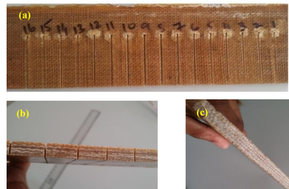
Fig. 3. (a) 16 cuts using AWJM (b) AWJM cutting (c) Saw cutting After machining, surface roughness (Ra) value of the machined surfaces were measured using Mitutoyo surfstest SJ210 model
