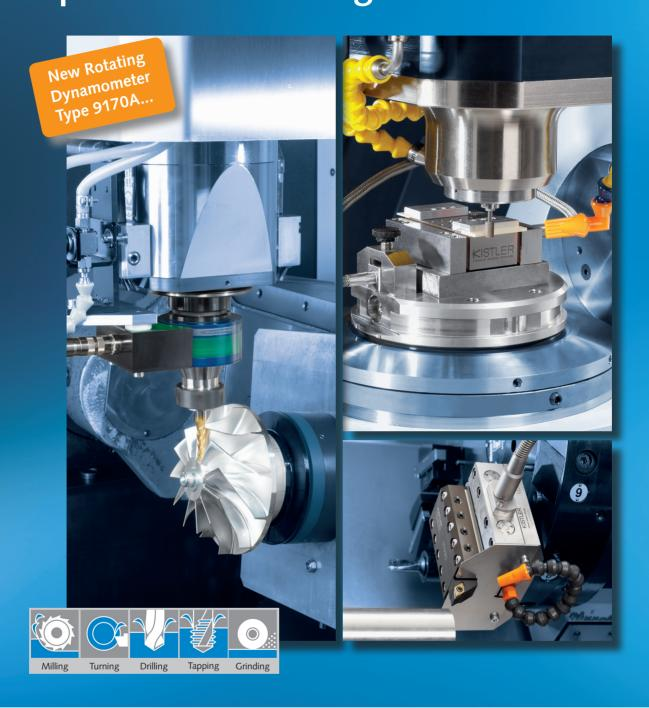
Analysis of mechanical loading of the tool cutting is very important in achieving integrated optimization of cutting processes. Piezoelectric dynamometers from Kistler provide reliable information about the level of forces and torques involved. Precise, highly responsive recording of these signals allows targeted improvement of all of the
